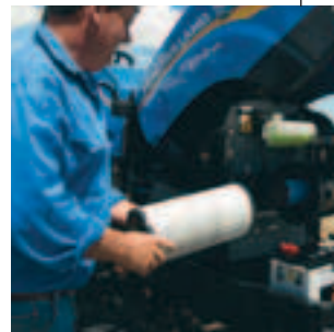
The air filter is easy to check, clean or replace with no need for tools.
