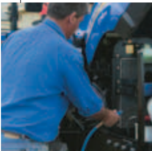
The cooling package slides out for simple and efficient cleaning.
