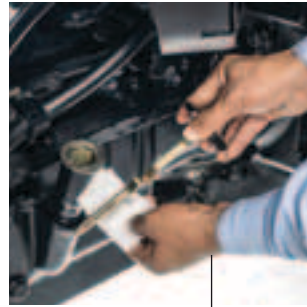
Engine and hydraulic oil are checked without opening the bonnet for faster checking and simpler servicing.
