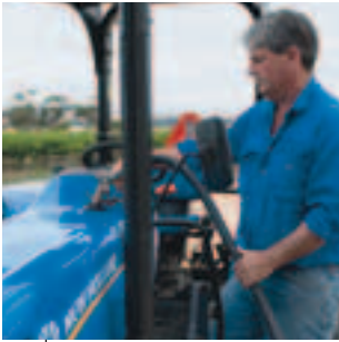
Refill the lockable 60 litre fuel tank from ground level.
